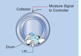
A low voltage current is passed through the laundry by specially insulated lifters. The moisture is measured 400 times per second.
